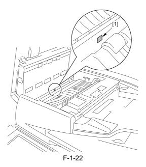
⚠ The surface of the prism coming in contact with paper is covered with plastic film. Be sure to clean the film.
