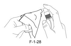
2) Apply the silicone oil to the reading glass [1] with the cleaning tissue.
