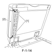
2) Clean the read roll [1] and the roll scraper [2] with lint-free paper moistened with alcohol.
