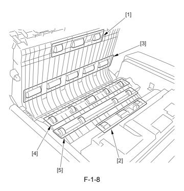
2) Clean the feeder inside cover [1], feed guide [2], reversing guide [3], delivery guide [4], and registration guide [5] (including sheets) with lint-free paper moistened with alcohol.
