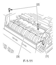
4) Clean the red roller 2 [1] and the read roller [2] with lint-free paper moistened with alcohol.
