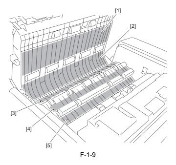
3) Remove the feeder cover and the feeder inside cover; then, clean the roll scraper [1] with lint-free paper moistened with alcohol.
